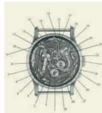
This drawing in the 1948 instruction manual for watchmakers, details the procedure followed when disassembling and assembling a perpetual calendar movement. The calendar requires no manual adjustment and is also programmed for February 29 of a leap year.
