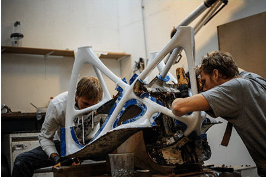
The present model armchair being removed from its mould Photo: Adriaan de Groot
