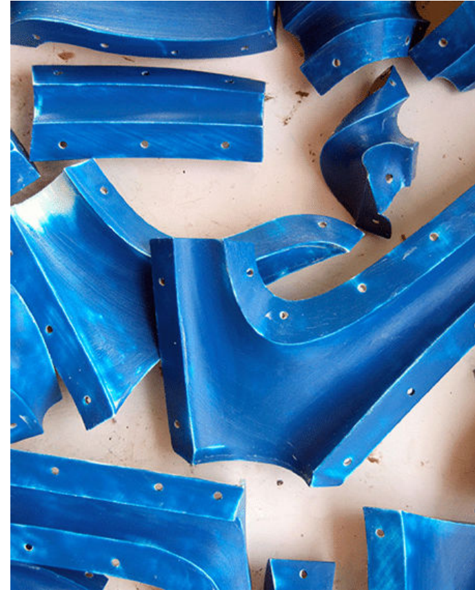
Close-up of the components of the armchair's 91-part mould Photo: Joris Laarman Lab
